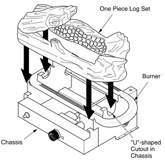
Figure 27 - Installing One-Piece Log Set
